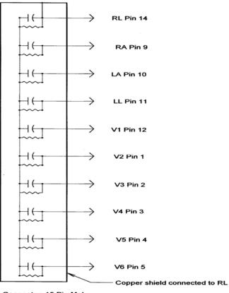
Connector: 15 Pin Male Resitors: All resistors 51K Ohm, 1/4 Watt, 5% Capacitors: All Capacitors 0.047 uF, 50 V, 10%
