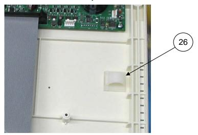
Apply 2 pieces of double sided tape (Item 23) to the Battery (Item 1), as shown. Note that the battery terminals are to the operator's right in this view.
