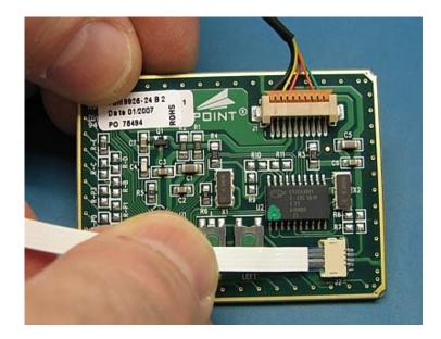
Insert the Touch Pad electronic assembly into the Keyboard Bezel in the orientation shown. Apply 2 pieces of Anti-Static Tape to retain the touch pad electronic assembly to the bezel during the assembly process.
