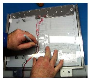
Cut 2 pieces of double sided foam tape (Item 35) approximately 6.5 to 7.0" in length and apply the tape to the backside of the Backlight Inverter Module PCB (Item 9) as shown.
