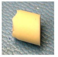
Insert the Elastomeric Plugs in the top two (2) screw hole of the rear housing. Ensure the plugs are flush to the housing. Note: the beveled side of the plug must match the bevel of the rear housing.
