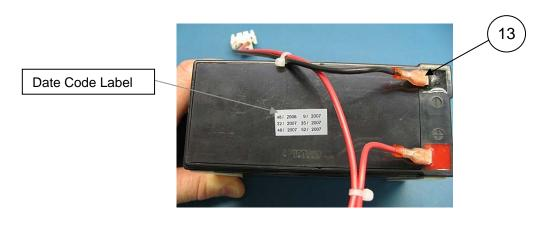
Remove paper backing from double sided tape and install battery into the lower housing as shown. Note the orientation of the battery terminals to the fuse holder.
