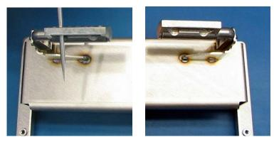
Note: Flat side of load plate must be up towards the rear housing.
