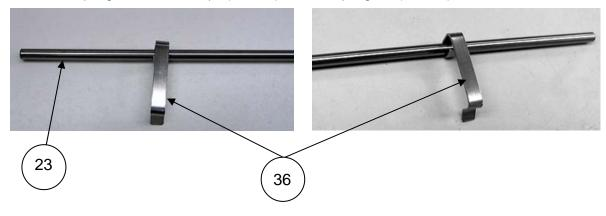
Slide the 2 spring bar retention clips (Item 36) over the spring bar (Item 23) as shown.
