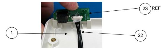
Route the tilt switch cable as shown using the rear housing as a guide. Retain the cable to the rear housing with tape (Item 29) 2 PIcs typical.
