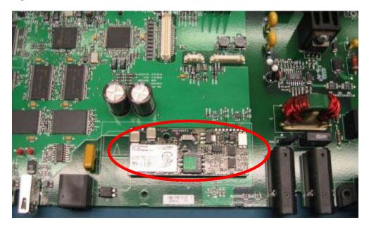
Figure 5-2 above shows the ELI 350 motherboard with the Modem option installed.
