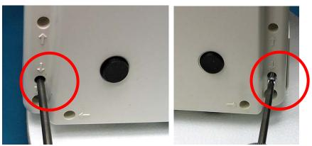
SNAP the Hinge Cover Housing to the Rear Housing. Ensure the LCD Monitor cables are not pinched between the housings.
