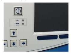
Apply the Keyboard Bezel Assembly to the Top Housing as shown. Ensure the bezel is centered in the opening.
