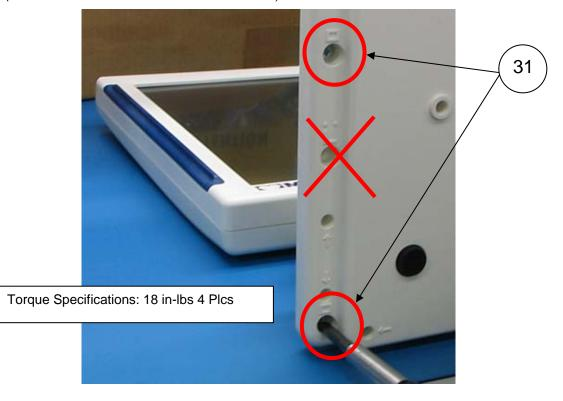
**NOTE**: 2 locations are circled for reference only. DO NOT use the location marked with an X (REF: Location used to mount ELI 350 to Cart).
