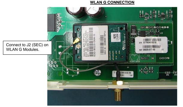
Press the Coax Cable (Item 5A) into the DPAC WLAN module connector J2(SEC) as shown until the cable is fully engaged as indicated by a click.
