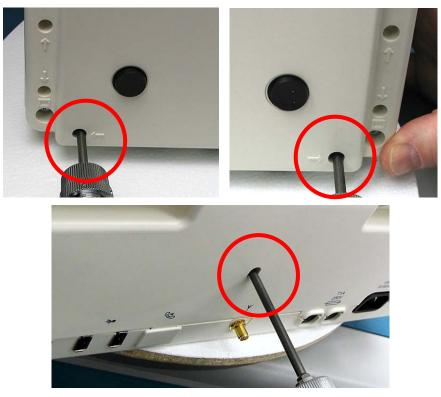
Insert silicon plug (Item 7) into the Rear Housing location. Note: The Arrow on the silicon plug must be UP.
