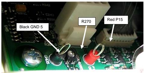
CRITERIA: Cue Sensor Settings: 2.0 VDC (Acceptable Range 1.90 – 2.10 VDC)
