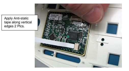
Feed the USB Cable and the flex circuit through the opening in the Keyboard PCB assembly. Pull up on J2 connector ears (on Keyboard PCB) to open connector. Insert the flex cable into the connector. Push the connector ears down as shown.
