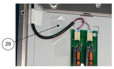
Insert the Backlight Inverter cable (Item 21) to the PCB Assembly. Route the cable as shown using the markings created on the LCD and retain the cable to the LCD with a piece of tape (Item 29)
