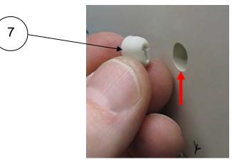
Open the LCD Monitor to assemble the Hinge Cover Housing (Item 4) to the Base Assembly.
