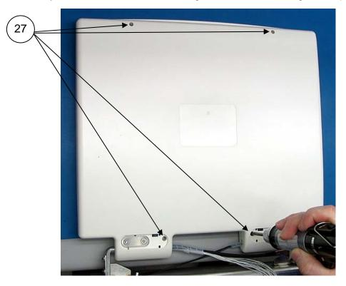
Flip the assembly over and fasten the Rear Housing to the Front Bezel using screws (Items 27, 4 Plcs).
