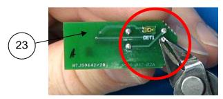
Connect the Tilt Switch cable (Item 22) to the Tilt Switch PCB Assembly (REF: Item 23) and insert the PCB into the display Rear Housing (Item 1) as shown.
