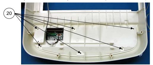
Retain USB cable to Top Housing using (part of the core BOM) using Cable Tie (Item 25) and Cable Tie Mount (Item 29).
