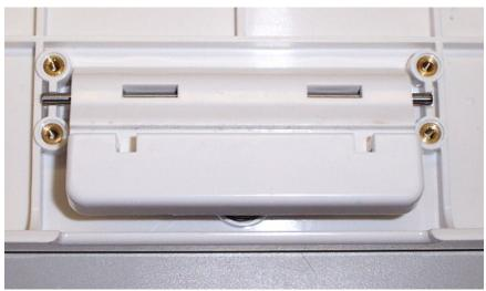
Place Latch Release with Pivot Bar installed onto Compression Spring as shown. Make sure Compression Spring sets in the spring capture area provided on Latch Release.
