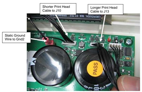
Connect the writer print head cables to the motherboard (longer cable to J13; shorter cable to J10). Connect the writer static ground wire from the writer to Gnd2 on the motherboard the motherboard.
