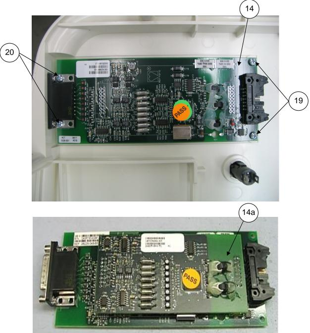
Install Front End PCB (Item 14) into Lower Housing and secure in place with 2 screws (Item 19) and 2 screws (Item 20).
