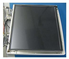
Assemble Front Bezel (Item 3) to the Rear Housing (REF: Item 1) using screws (Items 27, 4 Plcs).
