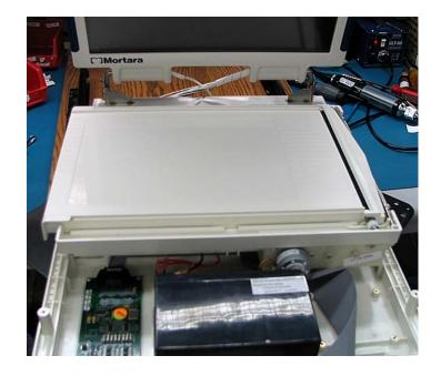
Install Writer Assembly (Item 10) – DO NOT rest the Writer Assembly directly on the motherboard.
