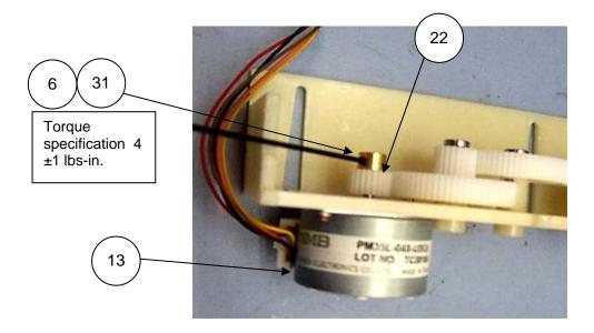
Prepare three Screws (Item 5) by brushing Vibra-Tite (Item 31) onto the threads as shown. Allow to dry for a minimum of 10 minutes. Note: This step may be done prior to assembling the unit so the Vibra-Tite has time to dry and the screws are ready to install. If the parts already have Vibra-Tite on the threads this step can be skipped.
