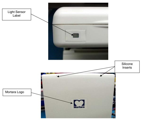
Silicon Inserts 2 plcs on rear of LCD display
