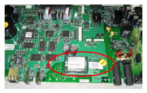
Figure 5-1 above shows the ELI 350 motherboard with the Wireless LAN option installed.
