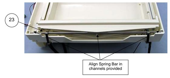
Snap the Retention Clips to the writer tray as shown. Open and close the writer cover drawer to verify proper operation ensuring there is no interference with the retention clips.
