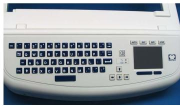
Flip the assembly over and secure the keyboard bezel to the top cover with 6 screws (Item 20).
