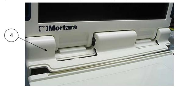
Secure the Hinge Cover Housing to the Lower Housing using 2 screws (Item 21).
