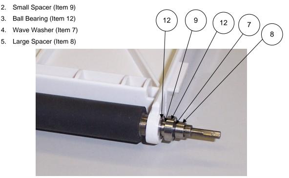
Lock the previous items in place with an E-Ring (Item 10) as shown. Make sure E-Ring snaps completely into the slot on the shaft.
