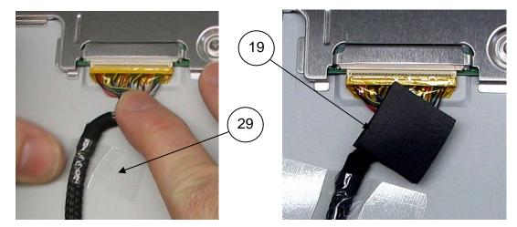
Apply LCD support block foam (Item 19) to retain signal cable top to the LCD.
