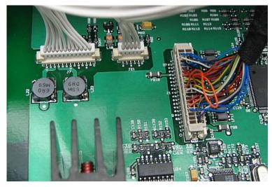
Connect LCD display cables (Qty 3) to the Motherboard as shown. Ensure cables are fully seated **NOTE**: All cables are keyed.
