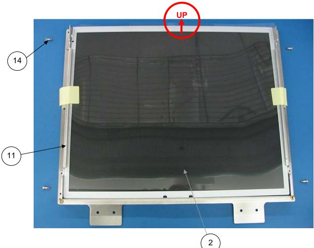
Flip the assembly over to mark the cable routings and backlight PCB location. Use caution not to damage the front of the LCD.
