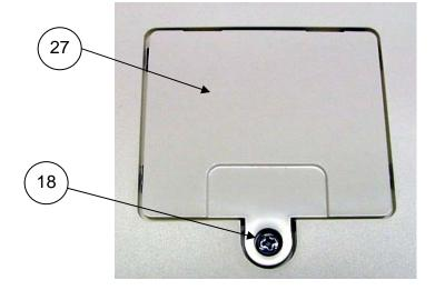
Insert the SIM Card Access panel (Item 27) into the Lower Housing and secure with screw (Item 18).
