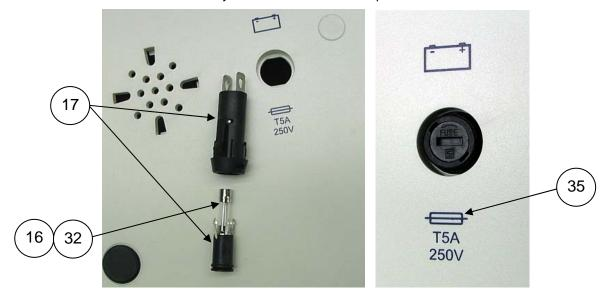
**IMPORTANT** – The battery fuse on the ELI 350 unit is dependent upon the item number of the unit's motherboard. Units manufactured with the older motherboard (Item #26025-076-51) use a 5A fuse; and those manufactured with the newer motherboard (Item # 26025-076-52) use an 8A fuse. Fuse labeling shown above is for the 5A fuse application; fuse rating labels (Item # 35) are available to properly label the unit chassis if a fuse rating change is required, due to a motherboard service replacement.
