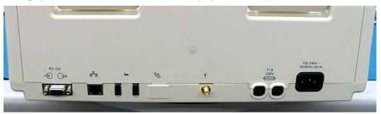
Antenna shown here connected for test purpose only. Disconnect the antenna to ship along with the unit. (fuse ratings pictured below are from a unit with display # 5400-016)
