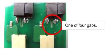
Remove the backing from the double sided tape and mount the Backlight Inverter Module PCB to the LCD centering within markings
