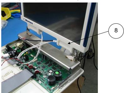
Place the LCD Display Sub-assembly (Item 8) on the Lower Housing as shown.
