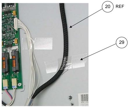
Cut a piece of 3/8" spiral wrap (Item 32) 4 inches long. Capture both the LCD Backlight cable and LCD Signal Cable within the spiral warp as shown.
