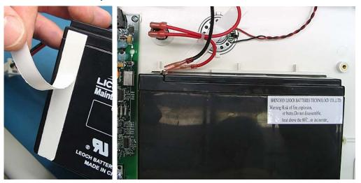
Connect battery cable to the fuse holder and Motherboard as shown.
