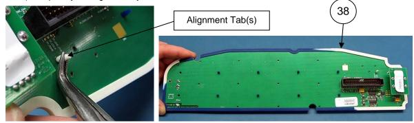
Apply Keyboard Bezel (Item 39) over the Elastomeric Keypad as shown. Ensure all keys extend through the applicable opening.
