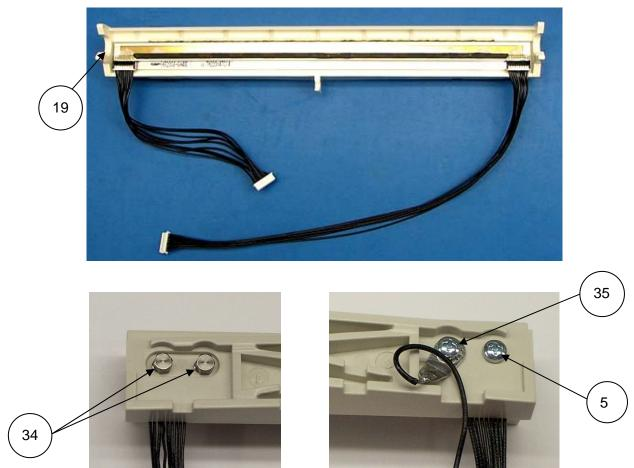
Place Print Head into Print Head Mount (Item 19) and secure with two shoulder screws (Item 34) and screw (Item 5). Attach ground wire (Item 28) with screw (Item 35) as shown.
